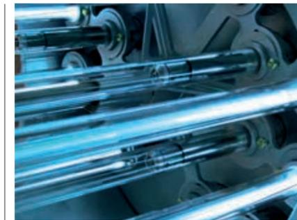
Ultraviolet light used to break down contaminants in water.
